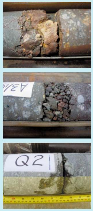
Recovered Cores displaying Pile Toe Interfaces of Varying Condition
