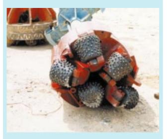
A Reverse Circulation Drill (RCD) Drilling Head
