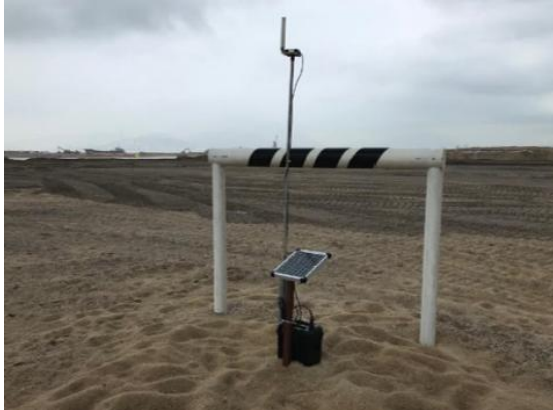
Figure 25 Permanent DGPS Station to Monitor Settlement Marker.
