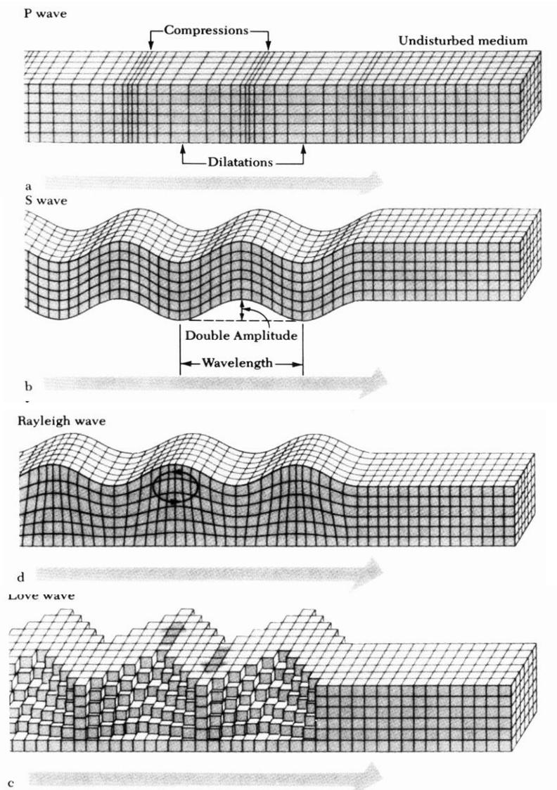
Rayleigh wave vibrates both vertical and horizontal direction.
