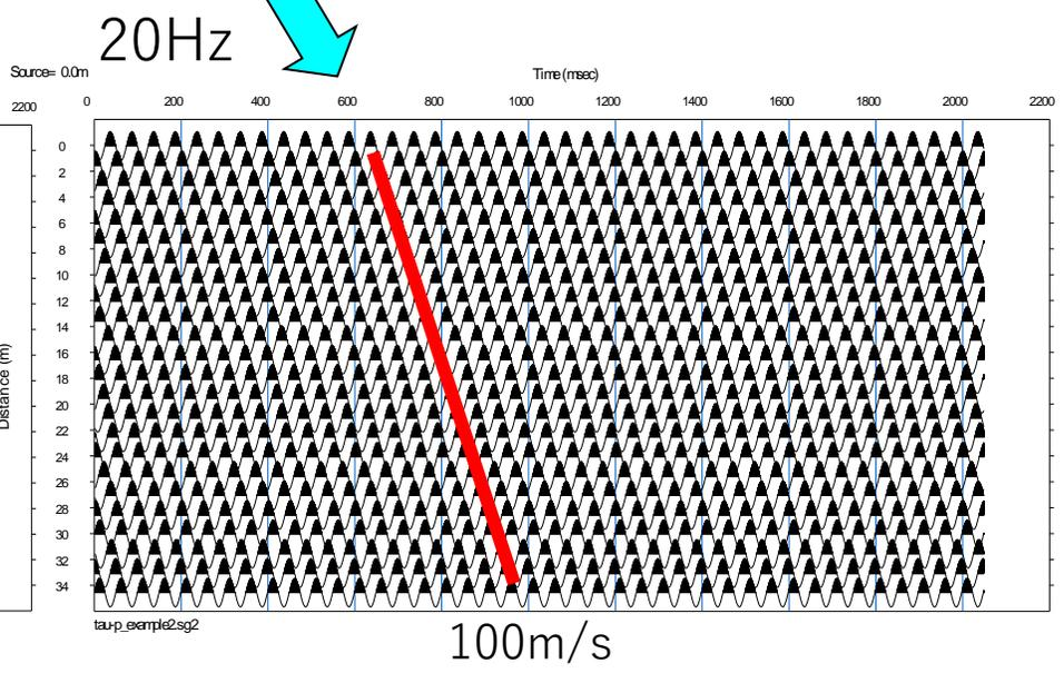
Monitoring S-wave velocity of the ground using continuous seismic ambient noise measurements
