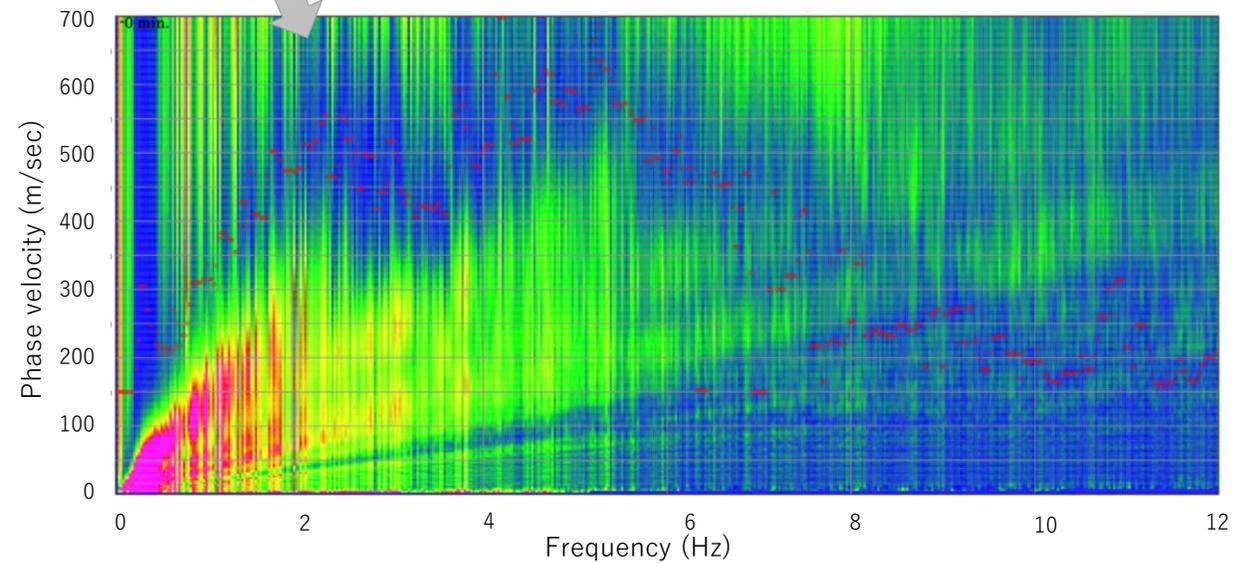
Monitoring S-wave velocity of the ground using continuous seismic ambient noise measurements
