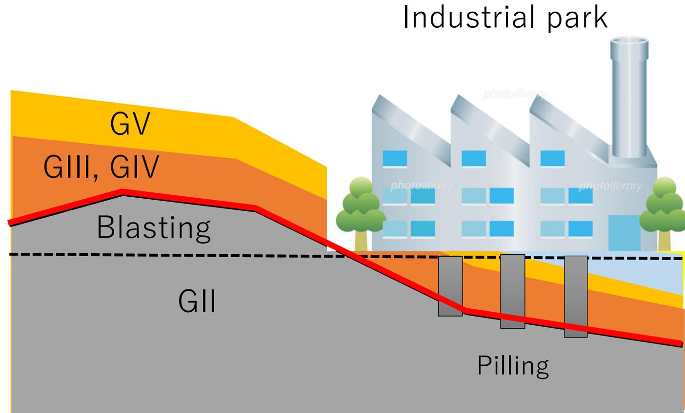
Delineate the depth to GII to estimate volume to blast and length of piles
