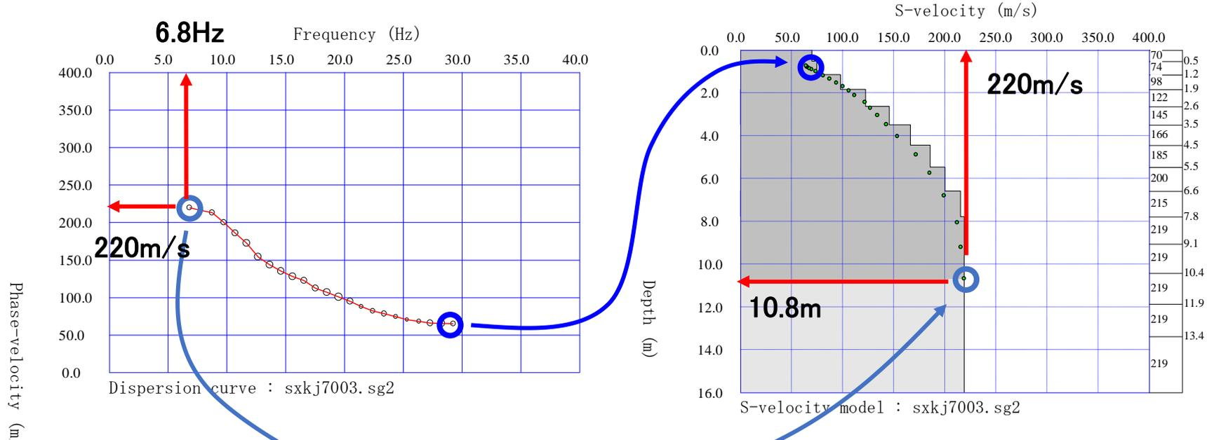
$$\text{Depth} = 10.8 = 220 / 6.8 / 3 = \text{Phase-velocity} / \text{Frequency} / 3$$
