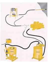
The electronic data Figure 7: Grouting Equipment for One Grout Line recording device gets
