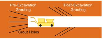
Figure 2: Pre- and Post-Excavation Grouting
