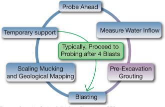
Figure 1: Operation Cycle - Drill & Blast Excavation + PEG
