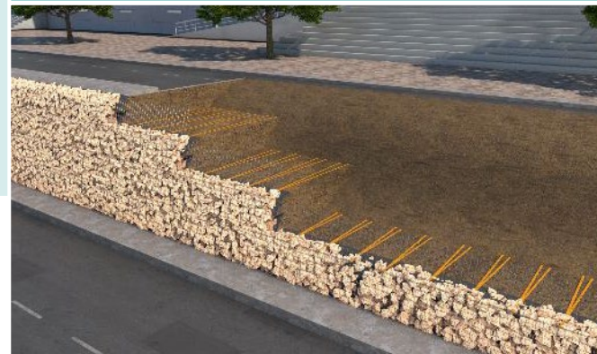
Mineral facing and geostrip reinforcement
