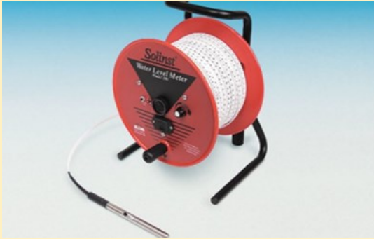
Fig 21 Observation Well/ Standpipe Piezometer Sensing Unit
