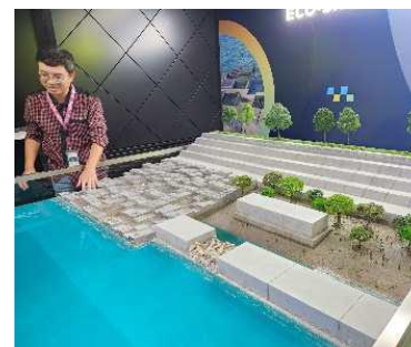
Small-scale model for each type of eco-shoreline design used in the project.
