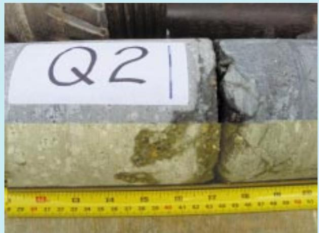
Recovered Cores displaying Pile Toe
