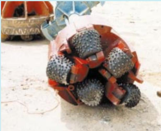
A Reverse Circulation Drill (RCD) Drilling Head
