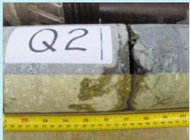
Recovered Cores displaying Pile Toe Interfaces of Varying Condition
